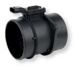
The mass air flow sensor measures the amount of air drawn into the engine and transmits this information to the engine control unit (ECU). This data is essential for adjusting fuel injection and ensuring an optimum air/fuel mixture, thereby ensuring efficient combustion, optimising engine performance and reducing pollutant emissions and fuel consumption.
