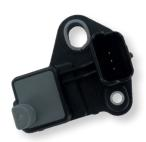
The crankshaft position sensor is an **essential electronic component of** the engine management system. It accurately measures the angular **position and rotational speed of the crankshaft**, enabling the electronic control unit (ECU) to adjust the engine's operating parameters.
