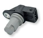
The camshaft position sensor measures the position and the rotational speed of the camshaft, a key factor in engine operation. It is used to synchronise fuel injection, regulate ignition, detect cylinder phase and activate variable valve timing.
