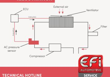
Air conditioning pressure sensors mainly use technologies based on pressure detection via mechanical or electronic sensors. The most widely used on the market is the mechanical diaphragm pressure sensor.
