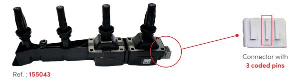
Primary winding resistance: approximately 0,5/1 Ω Secondary winding resistance: 11,3 KΩ
